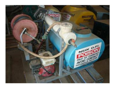
1x HONDA SPRAY UNIT KAPPA43/GX160 Spray unit comprising pump motor & 200 L stainless tank. Bait spraying unit (tank motor and pump).
